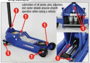
2 Trolley type Garage Jacks must be used on a smooth horizontal surface.
