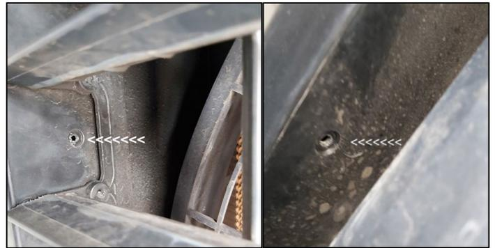
2. Remove the Automatic Diffuser and place on a bench with the outlet side facing upwards.
