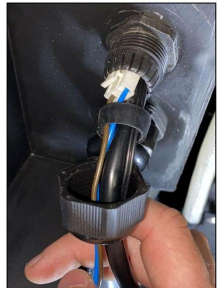
15. Connect the plug to the control panel and reconnect the yellow and green striped earth wire to the loom then loop the extra cable and Cable Tie it, tucking this behind the control panel. Refit the control panel with its screws.
