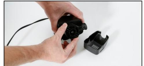
7. Twist the inner pump housing anticlockwise and remove from the main pump body.
