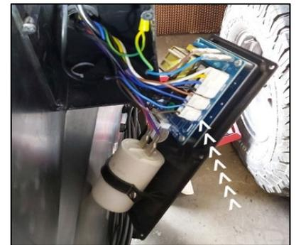
4. Disconnect the earth wire from the loom, note this is marked as a yellow wire with a green stripe. The earth wire can also be identified by the tag attached with earth symbol.
