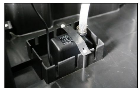
4. Remove the pump retainer and lift the pump from the base of the water tank.
