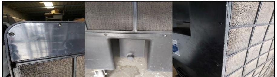
3. Thoroughly clean out the tank and ensure no debris is left in the pump and level float areas.
