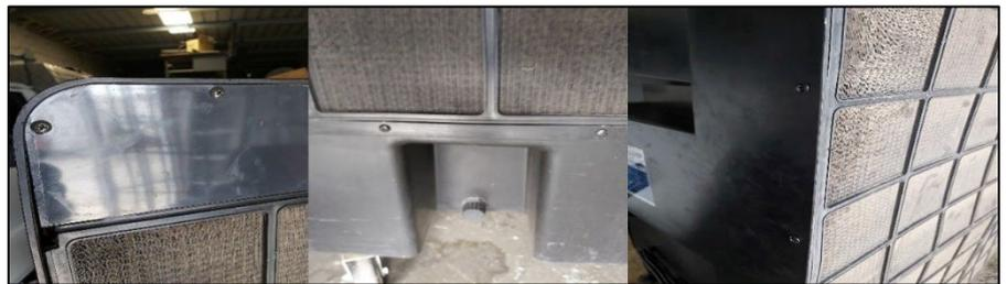
3. Remove the cooling pad and set aside.
