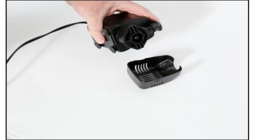
7. Twist the inner pump housing anticlockwise and remove from the main pump body.
